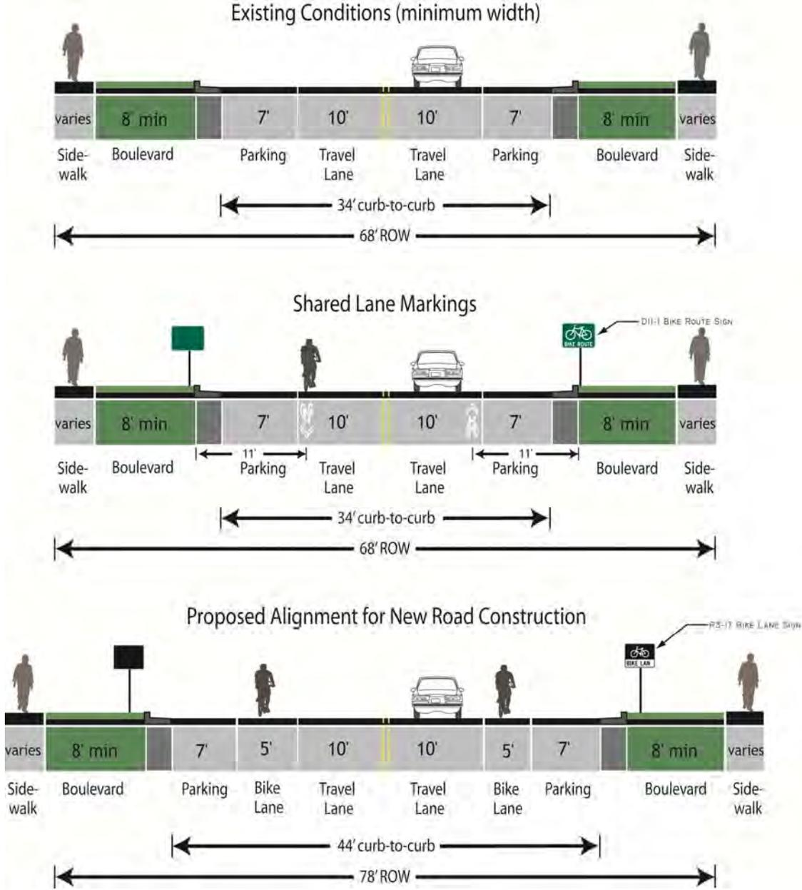
Figure 26. Alternatives for bicycle accomodation on collector roadways.
