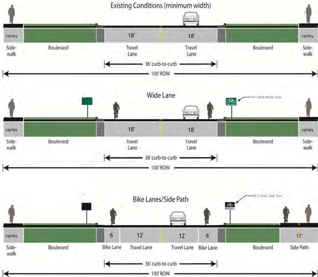
Figure 25. Alternatives for bicycle accommodation on arterial roadways.
