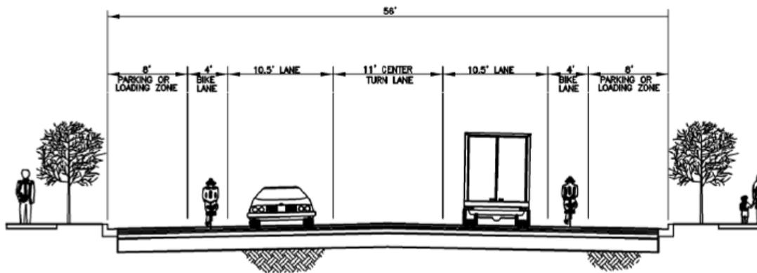
Figure 37. Proposed Highway 1416 Section with Bike Lanes.
