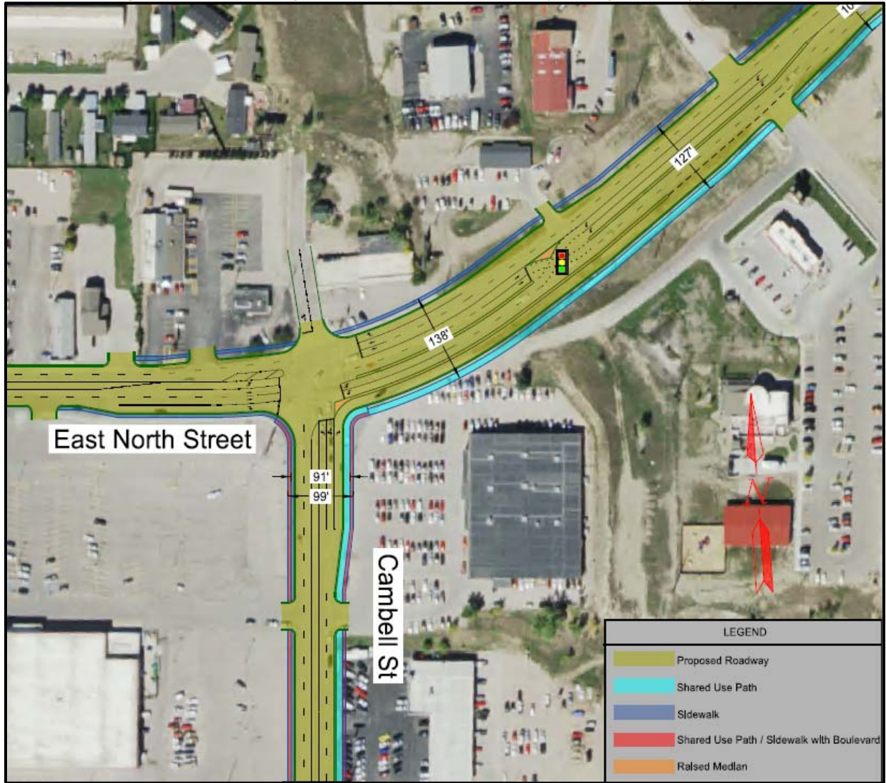
Figure ES.2 – Intersection of Cambell Street East North Street: Displaced Left Turns Configuration
