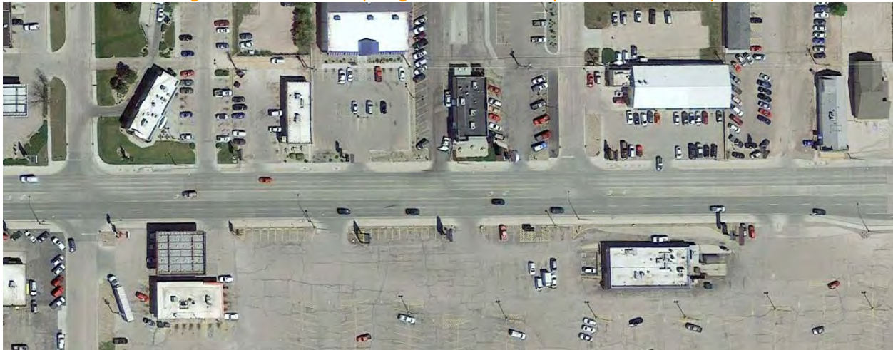
Figure 1.8 – Dense Access Spacing on East North Street (West of Cambell Street)
