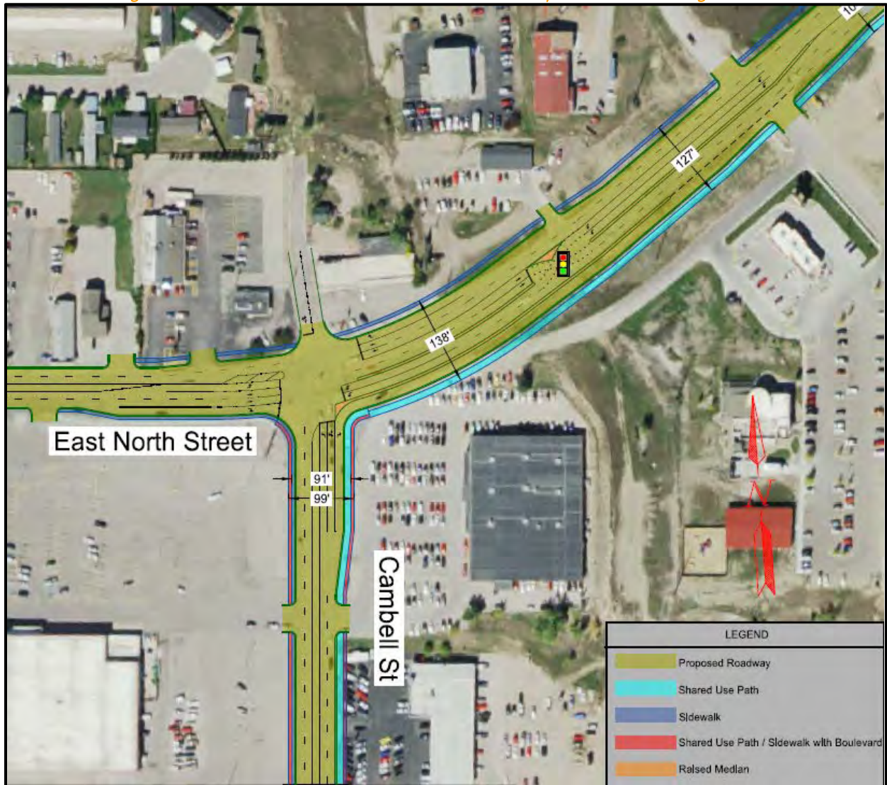
Figure 4.2 – Intersection of Cambell Street East North Street: Displaced Left Turns Configuration
