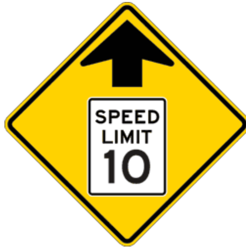
Figure 11 Reduce speed ahead sign
